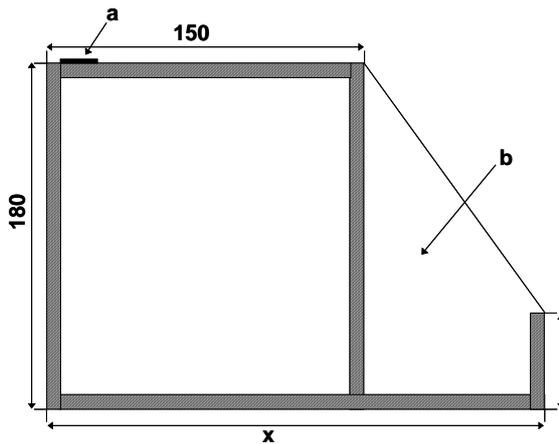
*Figure A.1. Side view of the apparatus for classification of accept chips according to length (or width).*
