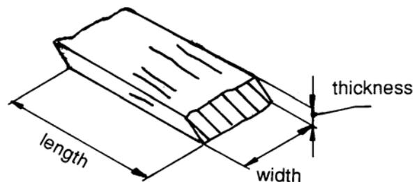
Figure 1. Sketch illustrating the definitions of the length and the width of an accept chip.
