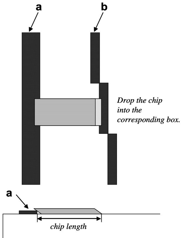
Figure A.3. Principle for chip length measurement.
