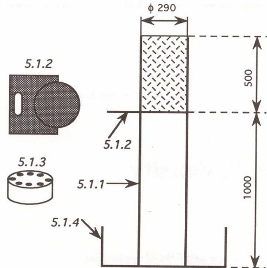
*Figure 1. Equipment for determination of the bulk volume of a chip sample:*
