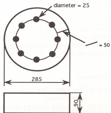
*Figure 2. Wooden lid (5.1.3), perforated with eight holes, dimensions in millimetres.*
