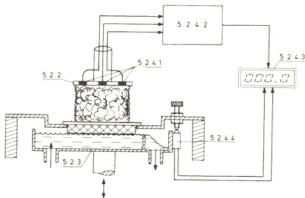
*Figure 4. Apparatus for determining the absorption time*
