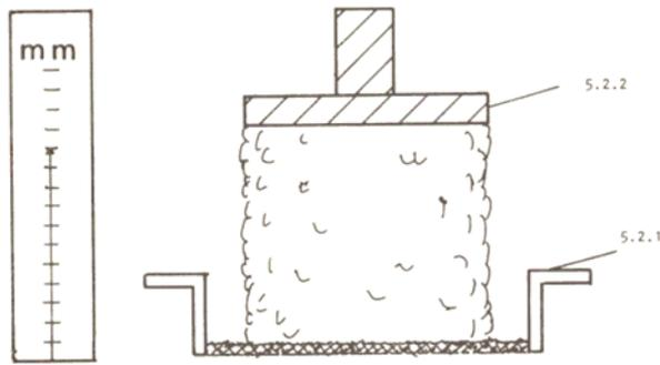
Figure 1. Determination of specific volume
