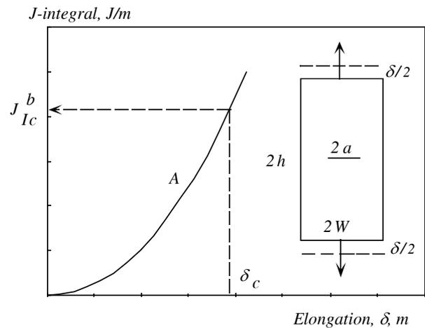
*Figure 1. From tensile test data, a J-integral-elongation curve (A) is constructed.*
