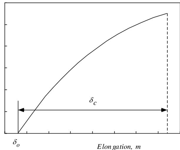
*Figure 3. Force-elongation curve for a fracture toughness test piece.*
