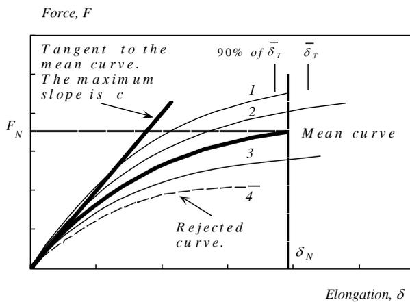
Figure 2. Principle for calculating properties from the tensile test.
