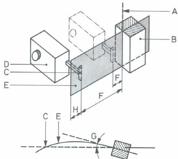
Figure. Principle of the bending resistance tester.
