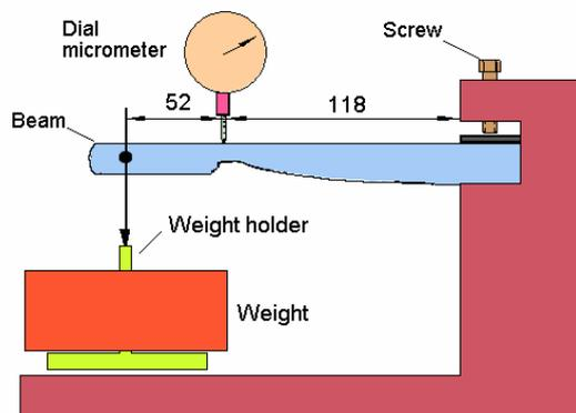
*Figure A.1. An illustration of the calibration procedure.*
