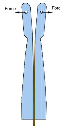
*Figure 2.* Measurement carried out by loading the beams horizontally.
