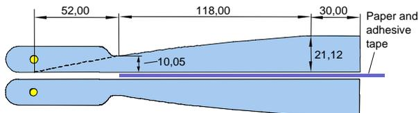
*Figure 1.* A pair of flexible beams. The dimensions, in millimetres, are theoretical values given with two decimals. For sufficient precision, a tolerance of  $\pm 0,05$  mm of these figures is considered to be enough.
