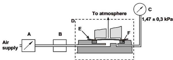
Figure 1. Principle of the Bendtsen tester
