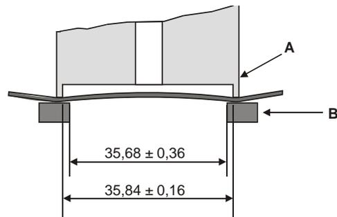
Figure 2. Dimensions of the measuring head (dimensions in millimetres)
