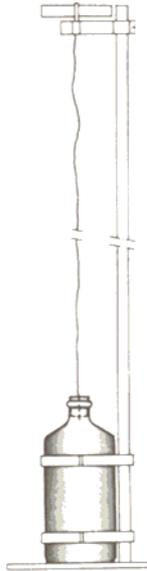
Figure 2. Sampling bottle for slurries.
