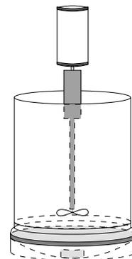
*Figure 1. A sketch of the fibre classifier*
