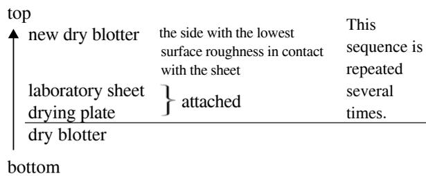
Place the stack in the press, raise the pressure rapidly to  $(400 \pm 10)$  kPa. Maintain the pressure for  $2 \text{ min} \pm 15 \text{ s}$  and then release it and remove the stack from the press.
