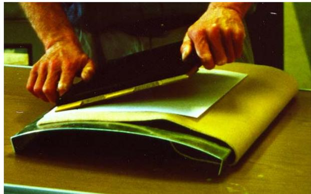
*Figure 1. A couching system comprising a curved plate covered with a felt.*
