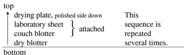
Place the stack of sheets centrally in the press (4.7) and raise the effective pressure on the sheets to  $(400 \pm 10)$  kPa continuously during 20 s to 30 s. Maintain this pressure for 5 min  $\pm$  15 s, then release it and remove the stack from the press.
